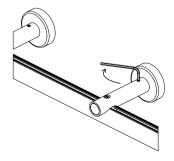
10. Slide the rail in the desired position and tighten all screws firmly.
