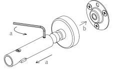
6. Loosen the screw so that the plate (c) comes loose.
